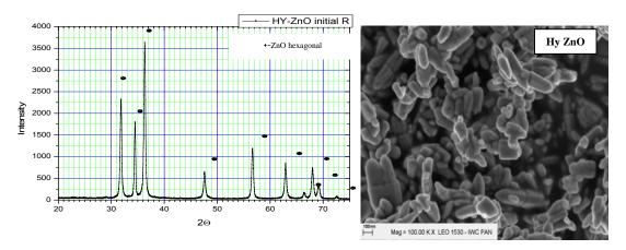
Fig.6. XRD Spectres of ZnO powders synthesized by hydrothermal route and the micrograph by SEM
